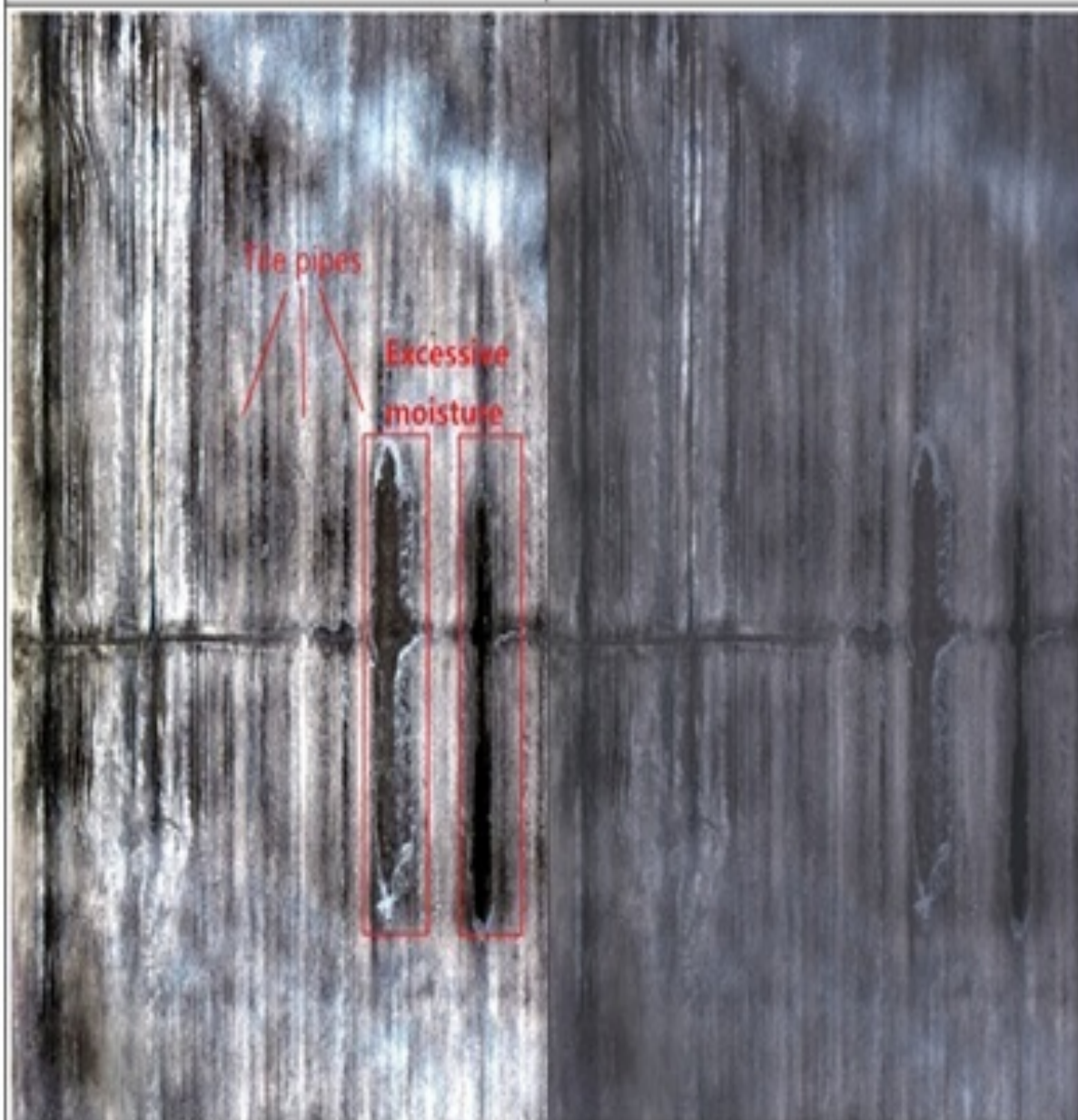
Fig. 8. Mosaicked image map for tile drainage pipes as captured by UAV
