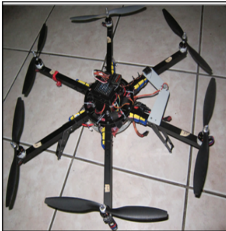
Fig. 2. Self-made UAV and its control deck
